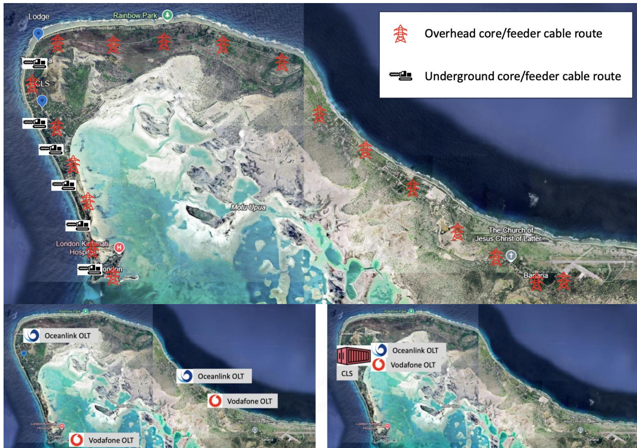
Figure 3.2b: Cable route and configuration and location of main links on Kiritimati
